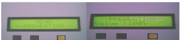
**Preheating menu** fixes the waiting temperature of the oven. The **A** button decreases, the **B** one increases the value, you validate with **C** button.
