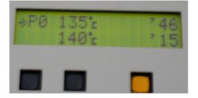
An arrow points the field, to modify it, press **C**, a star replaces the arrow, modify the value thanks to **A** button to decrease or **C** button to increase.
