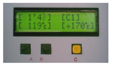
On the top: time and cycle phase (C1 preheating, C2 reflow and C3 cooling). On the bottom: probe value T0 (internal probe of the oven) and temperature consign for current phase.
